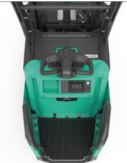
The series is available in foldable platform models with optional sidebars for use in narrow spaces, fixed platform rear entry models for fast operations where maximum operator protection is required, and fixed platform side entry models for easy on-off access on both sides for picking applications.
